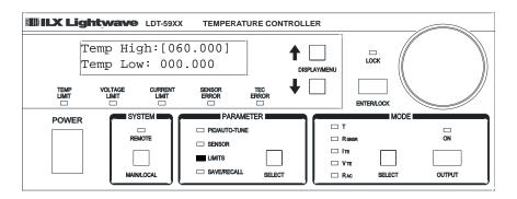
When these limits are exceeded, the corresponding LIMIT or ERROR LED in the Display Section is illuminated. Also, exceeding these limits may cause the controller output to be turned off automatically. (See the Output Off Registers section in Chapter 3).
