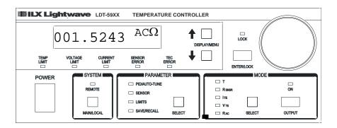
To activate this feature, press the OUTPUT key. The instrument will measure and display the resistance of the TE module, and then turn output off.
