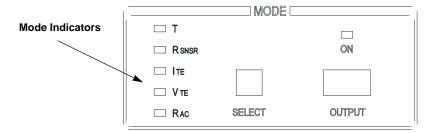
The OUTPUT key is used to turn the controller output current on or off. The OUTPUT is off when the instrument is first powered up. It may also be shut off automatically during operation if certain error or out of limit conditions occur. (See Chapter 3, "Output Off Registers"). Turning OUTPUT on enables temperature (or other mode) control of the TEC.
