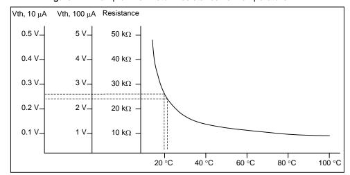
Figure 2.7 Example Thermistor Resistance vs. Temperature
