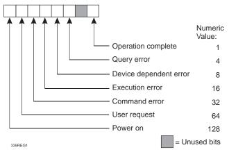
Notes Bit 5 of the the Status Byte Register (\*STB) is set if any enabled conditions are true.
