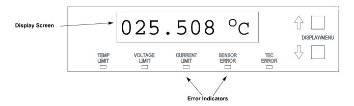
The error indicators (LEDs) in the display section are described as follows:
