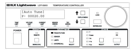
While Auto-Tune is in process, the PID/AUTO-TUNE LED will be flashing and the thermal system's temperature will be displayed. Once an Auto-Tune is complete, the instrument will then beep and disable the output, and the display will read "AutoTune Success". The instrument will automatically enter the new P, I and D values from a successful Auto-Tune.
