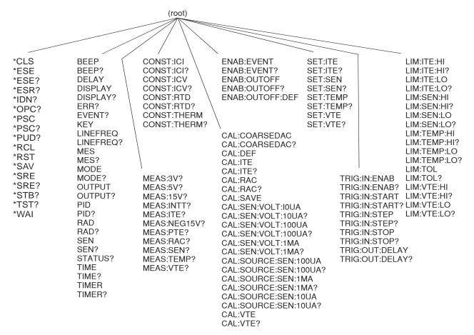
Figure 3.1 LDT-5900 Command Path Structure
