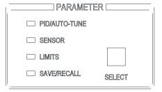
Parameter menu entry will automatically timeout after 10 seconds of no activity and the instrument will return to its default measurement display mode.
