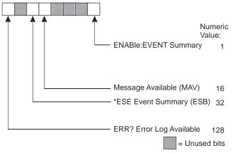
Notes Setting bits in this register enables GPIB Service Request (SRQ) generation. Example \*SRE 128 - Enables SRQ generation if the Error Log contains data (errors).
