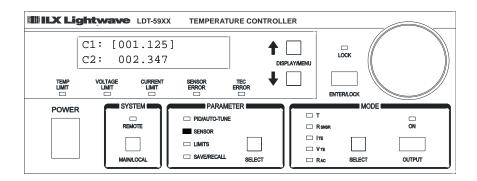
The coefficients can be modified by using the Adjust Knob and then pressing the ENTER / LOCK key. For more details on sensor, see "Sensor Options" later in this chapter.
